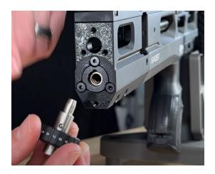
Replace power wheel not orientation of ball bearing that must match with the ball bearing groove
