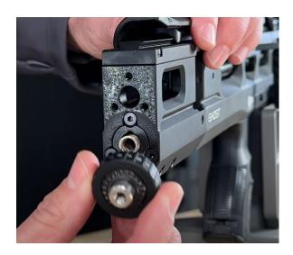
Remove spring and replace with spring of a different rating
