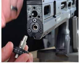
Replace power wheel not orientation of ball bearing that must match with the ball bearing groove.
