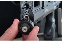
Remove spring and replace with spring of a different rating.
