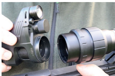
Rich prepares for the after-dark stage of his session by attaching the collar of the Pard NV007 to his scope and then coupling up the IR units bayonetted attachment.
