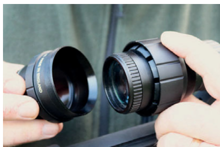
Rich prepares for the after-dark stage of his session by attaching the collar of the Pard NV007 to his scope and then coupling up the IR units bayonetted attachment.
