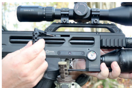
The sidelever Ghost's 300cc air bottle and Huma regulator meant Rich wasn't going to run out of shots.
