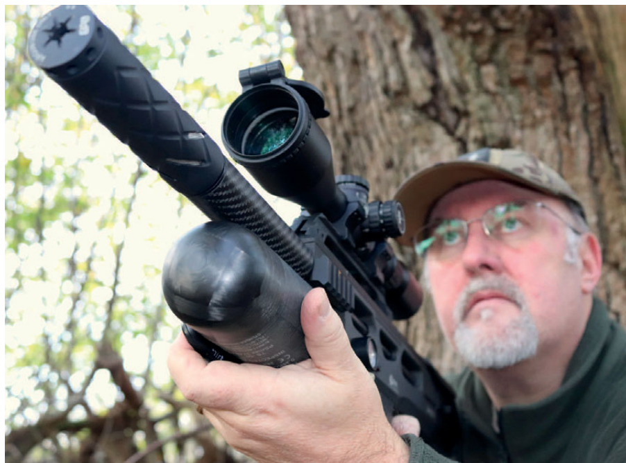
The sidelever Ghost's 300cc air bottle and Huma regulator meant Rich wasn't going to run out of shots.
