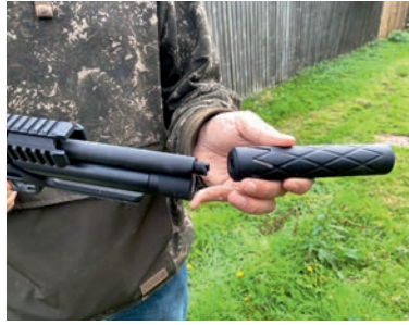
RIGHT: The shrouded barrel is threaded for a silencer
