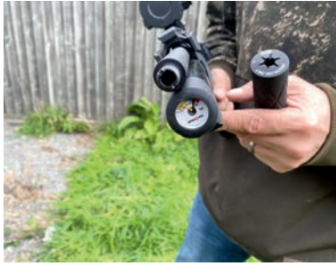
LEFT: The shroud at the end houses the fill gauge and fill port
