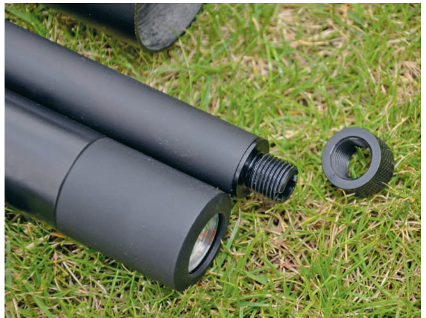
Detail of the threaded muzzle, note the manometer
