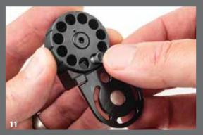
Open the front loading gate on the magazine and rotate the inner drum one rotation clockwise (figure 11)
