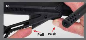
completely, push in the catch and at the same time pull the lever out as shown in figure 16. In addition, on Compatto 2 & XR the recoil pad may be adjusted for height to improve gunfit.
