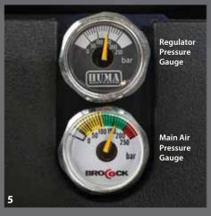
\*WARNING Do not attempt to adjust the regulator's pressure without first consulting a trained servicing agent, as to do so can irreparably damage the regulator seals and invalidate the warranty.
