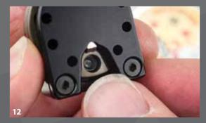
Rotate the magazine drum anti-clockwise to expose the next empty chamber and load another pellet
