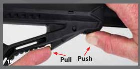
completely, push in the catch and at the same time pull the lever out as shown in figure 16.
