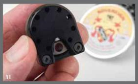
Press it in place fully, so that the pellet's head seats past the O-ring gripper and its skirt does not project
